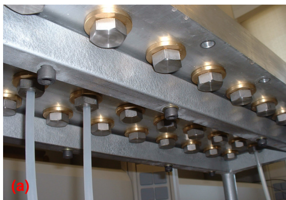
Figure 1.10 (a) Bottom view of the mold with 45 multi-function bolts; and (b) different uses of bolts.
