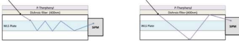
Figure 5.1. Comparison of the trapping mechanisms of the standard ARAPUCA (right) and the X-Arapuca (left). The X-Arapuca traps scintillation photons through total internal reflection, improving photon collection efficiency and enabling it to capture more scintillation photons than the standard ARAPUCA.
