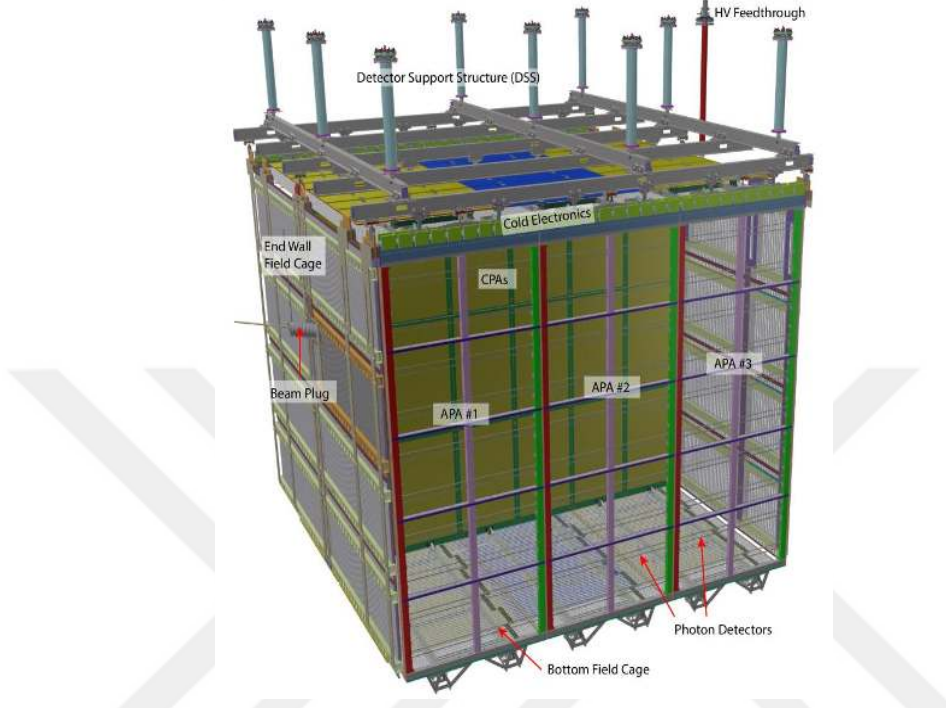
Figure 4.5. 3D model of the ProtoDUNE-SP detector with the labeling of all major components (B. Abi et al., 2020b).
