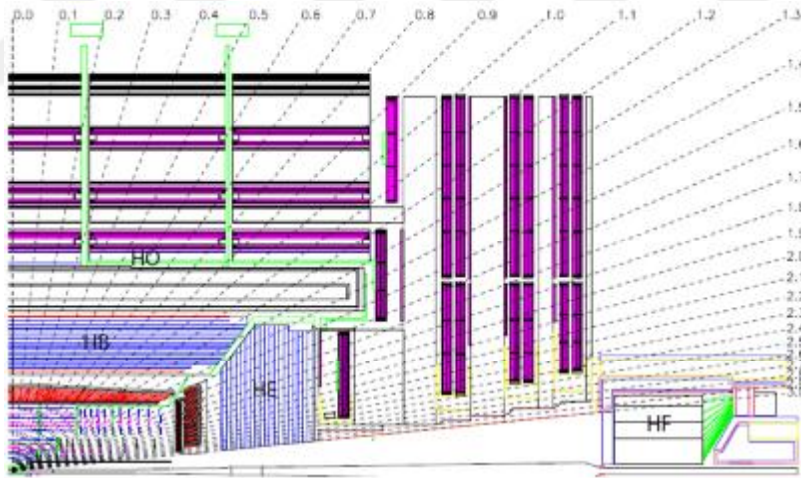
Figure 1.29. Longitudinal view of one quarter of the detector in the \eta - \phi plane, showing the positions of the HCAL parts: hadron barrel (HB), hadron outer (HO), hadron endcap (HE) and hadron forward (HF) (Chatrchyan et al., 2008a)
