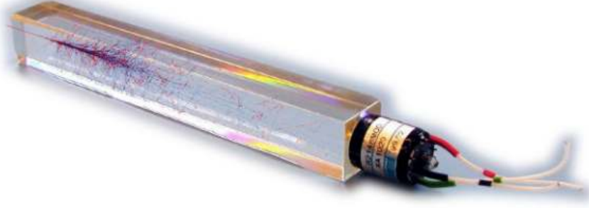
Figure 3.8. Image of a lead tungstate ( \text{PbWO}_4 ) crystal with an electromagnetic shower shown inside. Figure taken from (Wadud, 2019)
