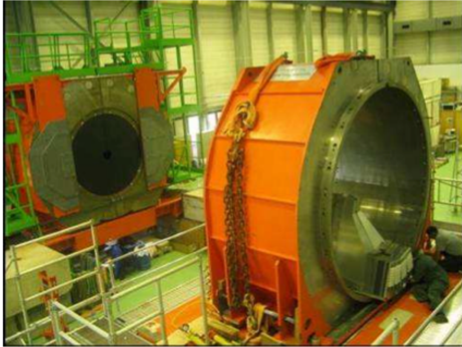
Figure 3.17. A fully assembled and a partially assembled structure of the forward hadron calorimeter (Banarjee, 2005).
