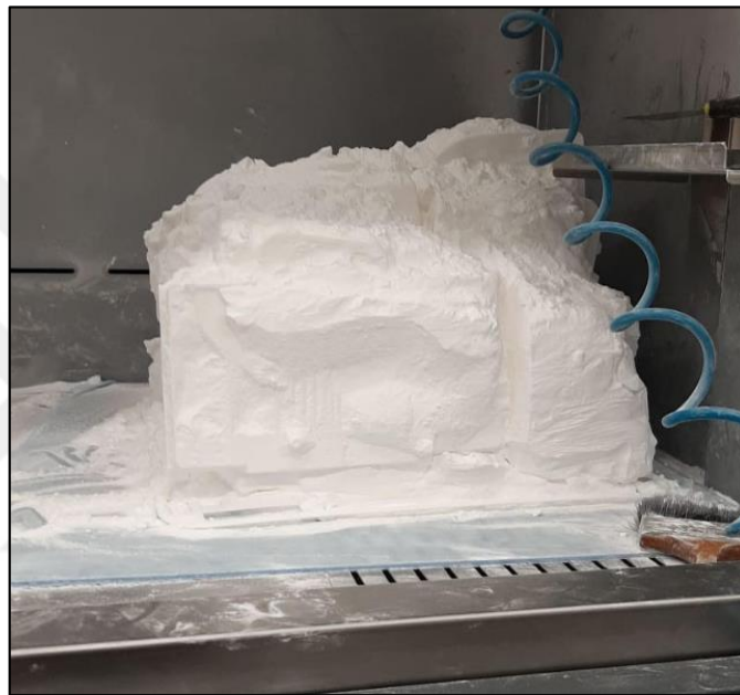
Figure 13 Cool-down stage at the end of the manufacturing process [source: Arçelik AŞ]
