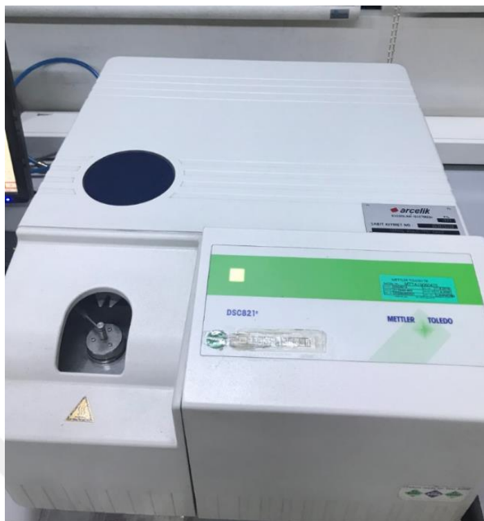
Figure 49 Mettler Toledo DSC821e, heat-flux type DSC
