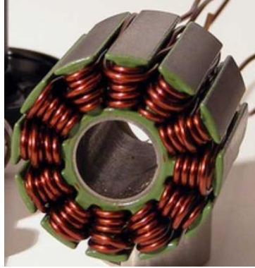
Figure 3.2. Concentrated stator windings.
