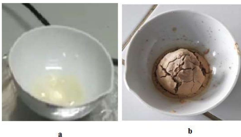
Picture 4.5 The images of \text{Zn}_3\text{B}_2\text{O}_6 samples for CA fuel a) gel form, b) synthesis
