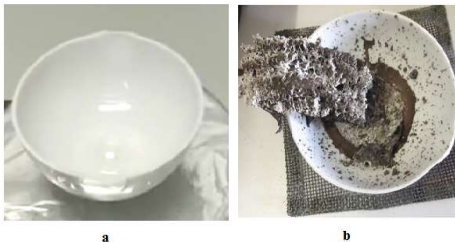
Picture 4.2 The images of \text{Zn}_3\text{B}_2\text{O}_6 samples for glycine fuel a) gel form, b) synthesis
