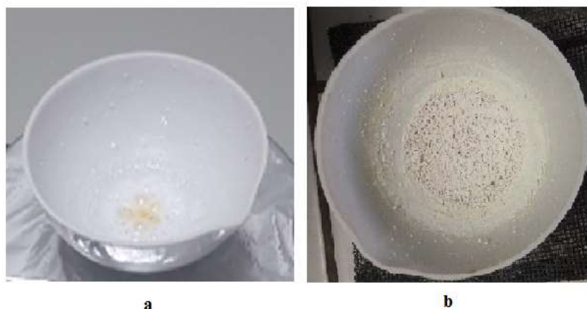
Picture 4.4 The images of \text{Zn}_3\text{B}_2\text{O}_6 samples for HMTA fuel a) gel form, b) synthesis
