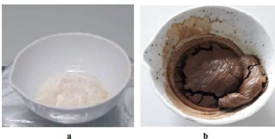
Picture 4.3 The images of \text{Zn}_3\text{B}_2\text{O}_6 samples for tartaric acid fuel a) gel form, b) synthesis
