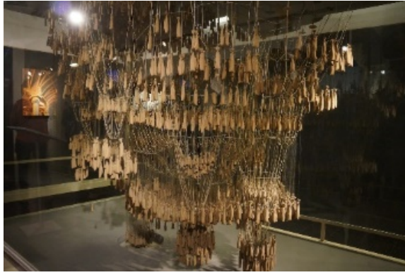
Figure 12. Gaudi, A., Hanging Chain Model [Photo]. ( http://dataphys.org/list/gaudis-hanging-chain-models/ 06.01.23)
