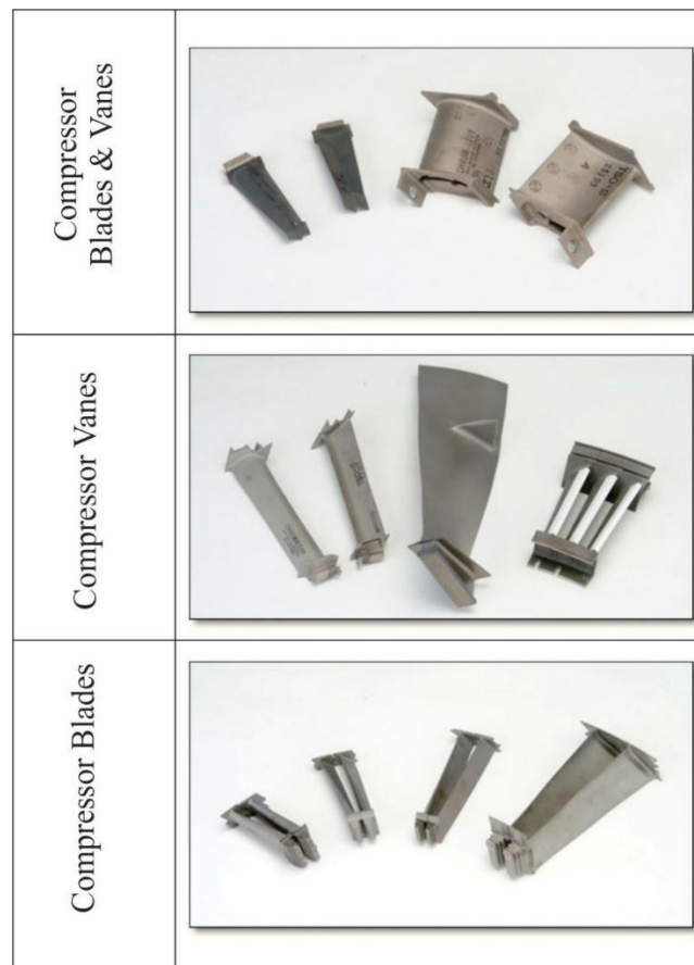
Figure 1-1 – Blades from Pratt &Whitney JT3D, JT8D, JT9D Engine families [2].
