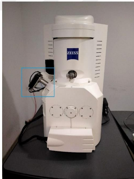
Figure 39 The image of the SEM system with EDX detector shown in the blue rectangle.
