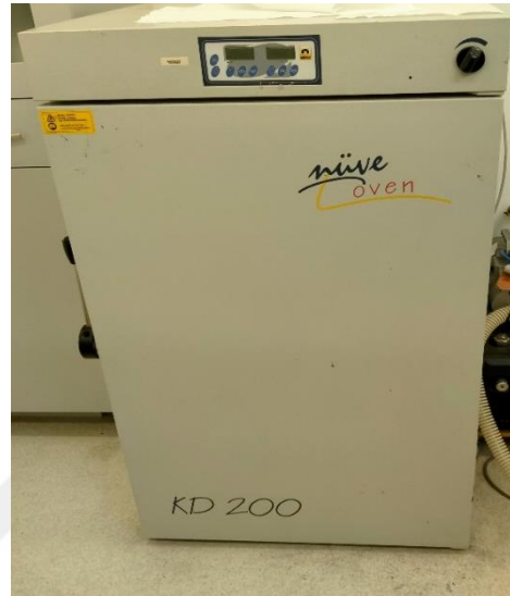
Figure 30 The image of the drying furnace.
