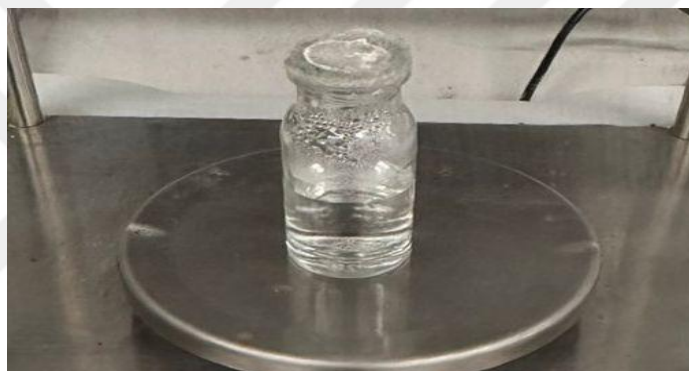
Figure 3.4: Water Vapor Transmission Rate Test.
