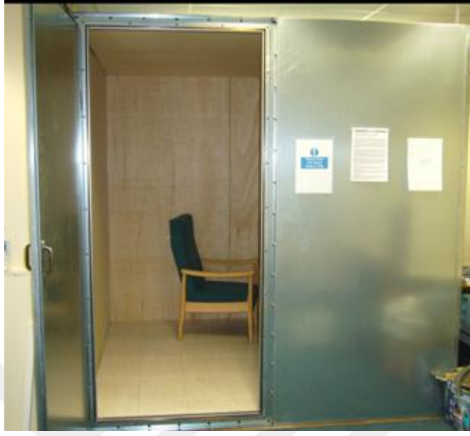
Figure 4.4: Sound proof room used for performing experiments
