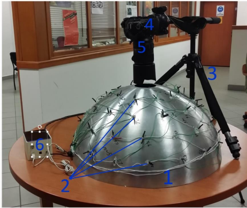
Figure 4.11 The RTI dome developed at Koç University Optical Microsystems Laboratory. The whole setup includes: 1. an aluminum dome of 30 cm radius, 2. 56 LEDs, 3. a tripod, 4. Nikon 7100 DSLR camera, 5. Nikon 105 mm macro lens, and 6. the electronics control unit with an Arduino Mega chip without any extra shielding.
