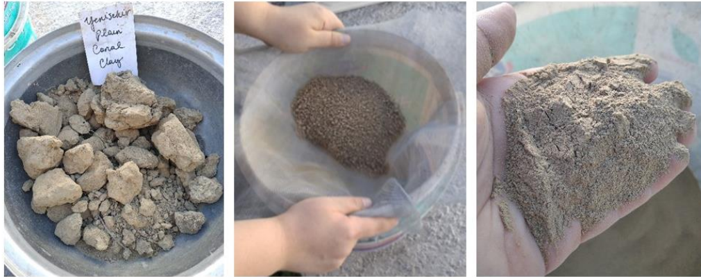
Figure 6.2 Marmaracık Lake Drainage Canal Clay before beating (left), sieving with a 1x1 mm grid sieve (middle), after sieving (right)
