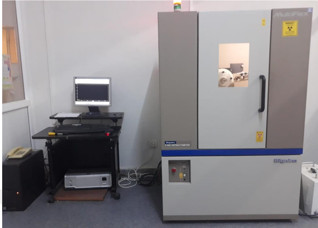
Figure 2.5. Rigaku Multiflex X-Ray Diffractometer in Physics laboratory.
