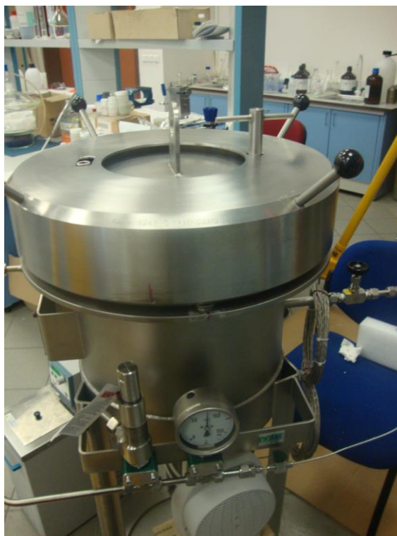
Figure 3. 17 Side view of Natex large scale extraction unit with cover, bayonet ring and safety plug
