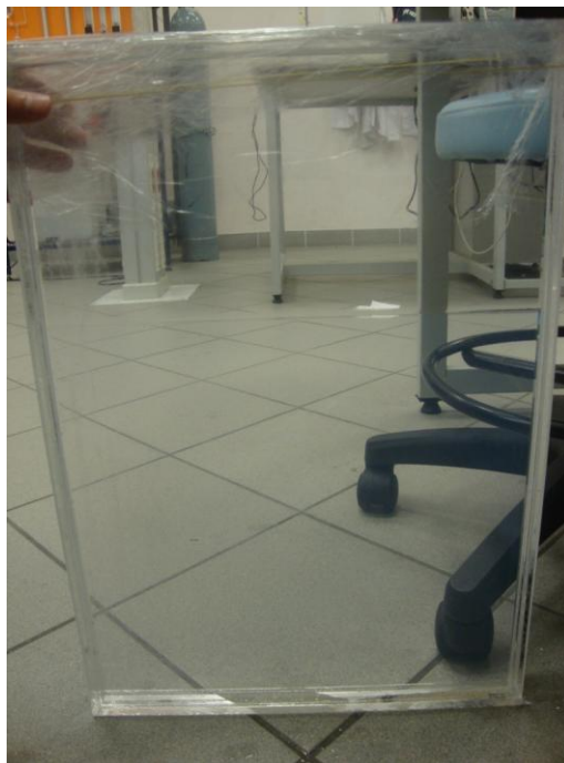
Figure 3. 13 Large scale plexiglass mold
