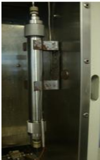
Figure 3. 11 Applied Separation smaller vessel in the oven
