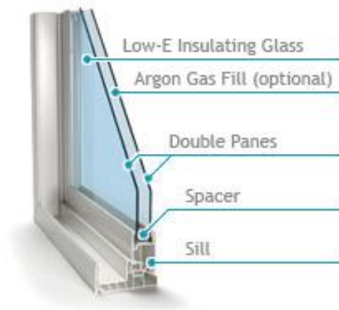
Figure 2. 2 A double window glazing system
