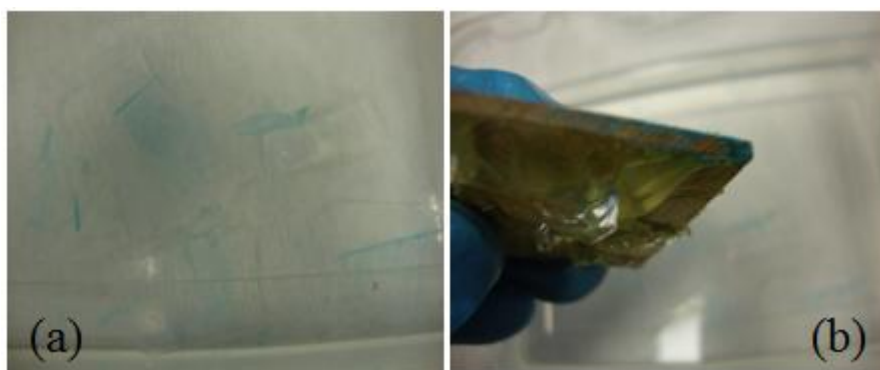
Figure A- 10 Effect of brass on surface of a PHP-Etac silica wet gel
