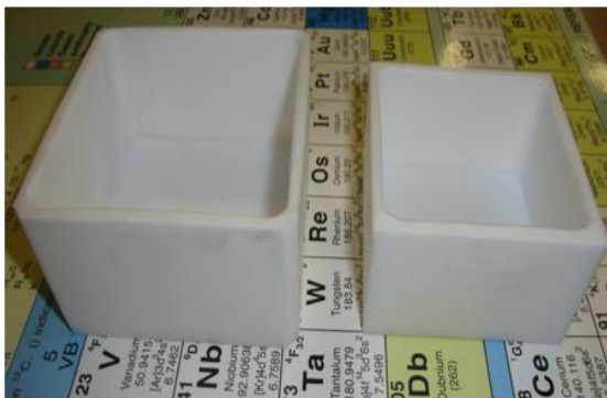
Figure 3. 3 Manufactured Teflon mold
