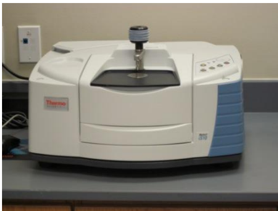
Figure 3. 21 Thermo Scientific Nicolet Avatar 360 E.S.P. FTIR spectrophotometer with Horizontal Attenuated Total Internal Reflectance (ATR) system
