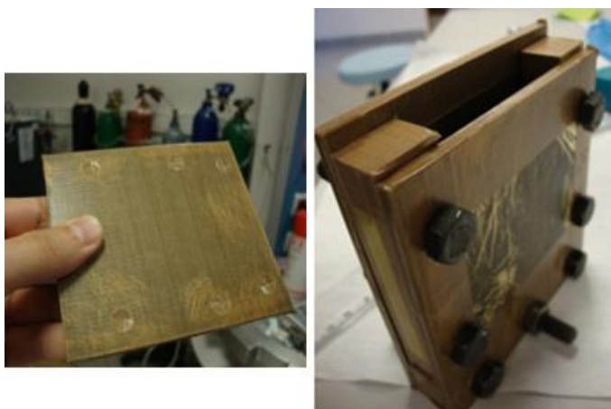
Figure 3. 6 Teflon film covered brass mold
