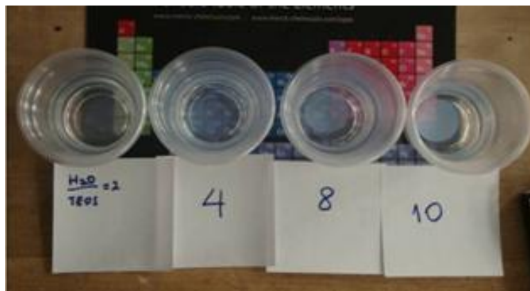
Figure 4. 3 Effect of W/T molar ratios on transparency of silica alcogels (E/T: 4)
