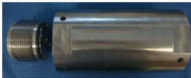
Figure 3. 12 Applied Separation larger extraction vessel (D: 7.5 cm and H: 12 cm)
