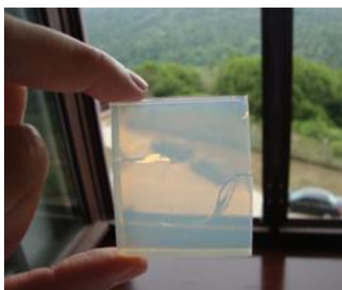
Figure 4. 35 Cracked silica aerogel aged in pure EtOH
