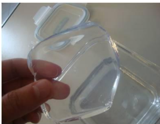
Figure 4. 31 Silica wet gel synthesized in a glass mold
