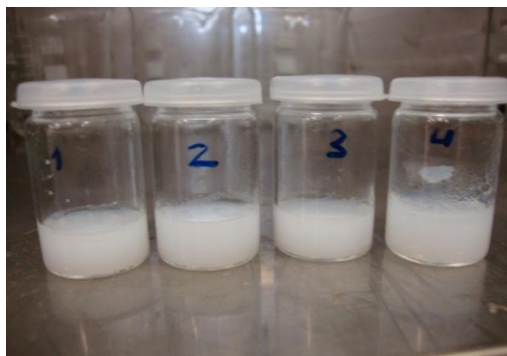
Figure 4. 1 Single step base catalyzed silica wet gels
