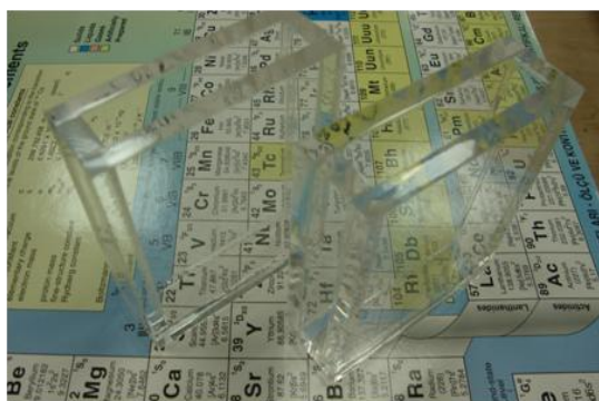
Figure 4. 34 Plexiglass mold with different shape to eliminate bending
