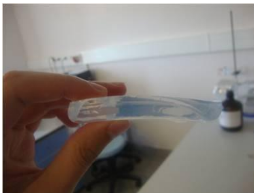
Figure 4. 32 Bended silica wet gel due to mold shape
