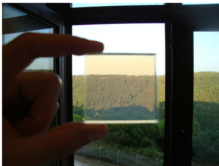
Figure A- 3 A silica aerogel with high transparency (TR%: 88) (E/T: 3 and W/T: 3)
