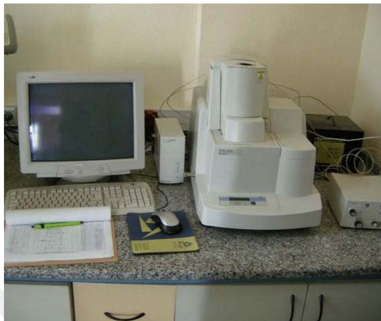
Figure 3.10 Perkin Elmer STA 8000 TG/DTA device (Personal archive, 2019)
