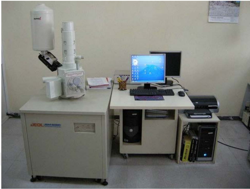
Figure 3.13 JEOL JSM-6060 model SEM device (Personal archive, 2019)
