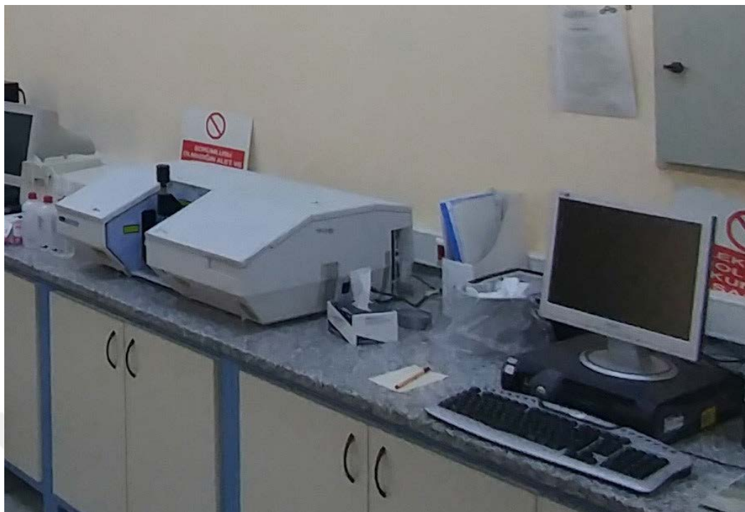
Figure 3.8 Image of the used FTIR device having ATR apparatus (Personal archive, 2019)
