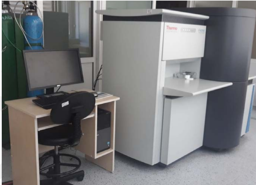
Figure 3.12 Thermo Scientific K-Alpha XPS device (Personal archive, 2020)
