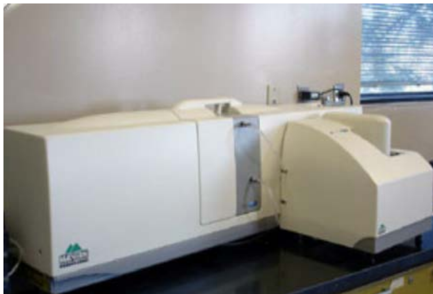
Figure 3.9 Malvern Zetasizer Nano ZS model device (Personal archive, 2019)
