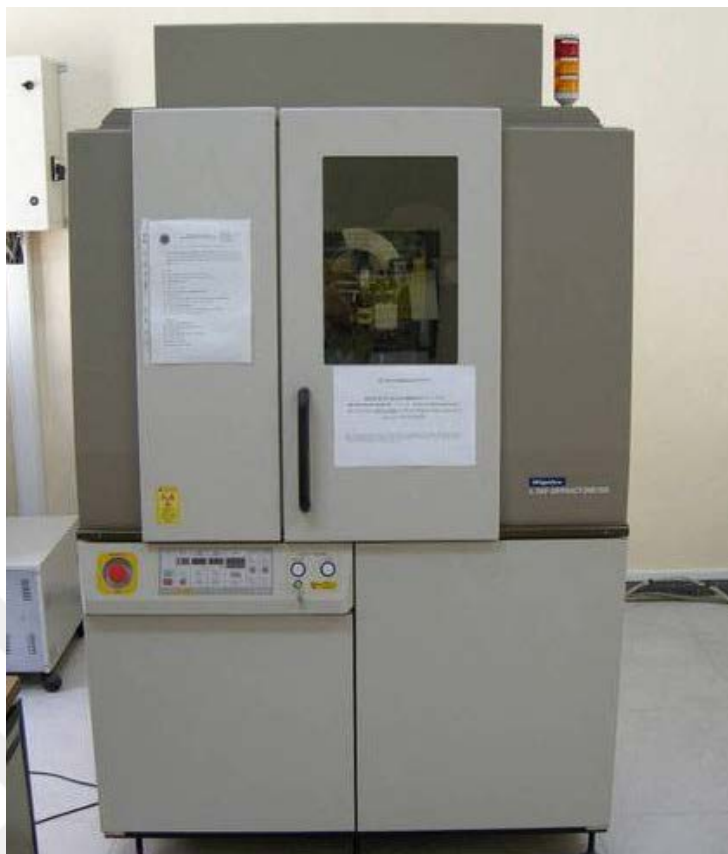
Figure 3.11 X-Ray Diffractometer, Rigaku, D/Max-2200/PC (Personal archive, 2019)
