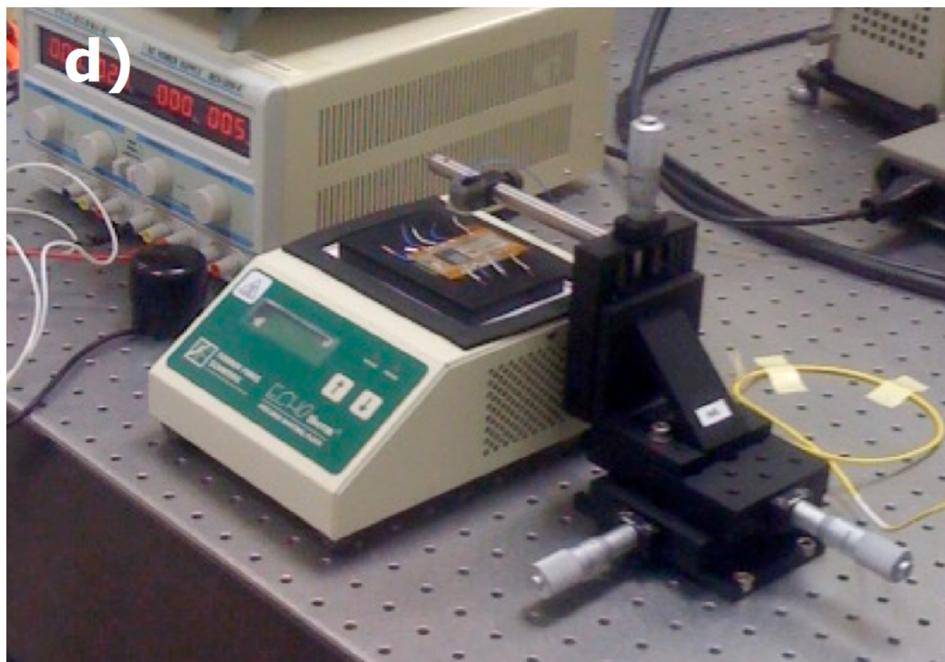
Figure 4.10 a) Schematic representation of optical characterization set-up and photograph of the b) general view of the set-up, c) light modulation part and d) fiber-to-detector coupling part
