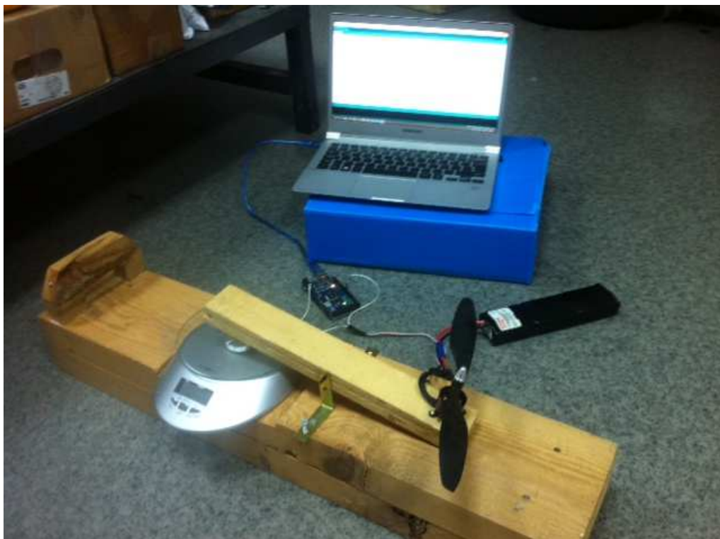
Figure 2.5 Test setup for simplified excitation models
