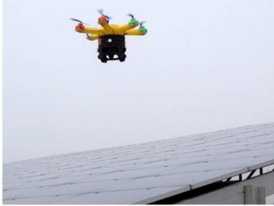
Figure 1.3 Nimbus UAV is monitoring PV Plant with thermal imagery and evaluates error conditions[5]
