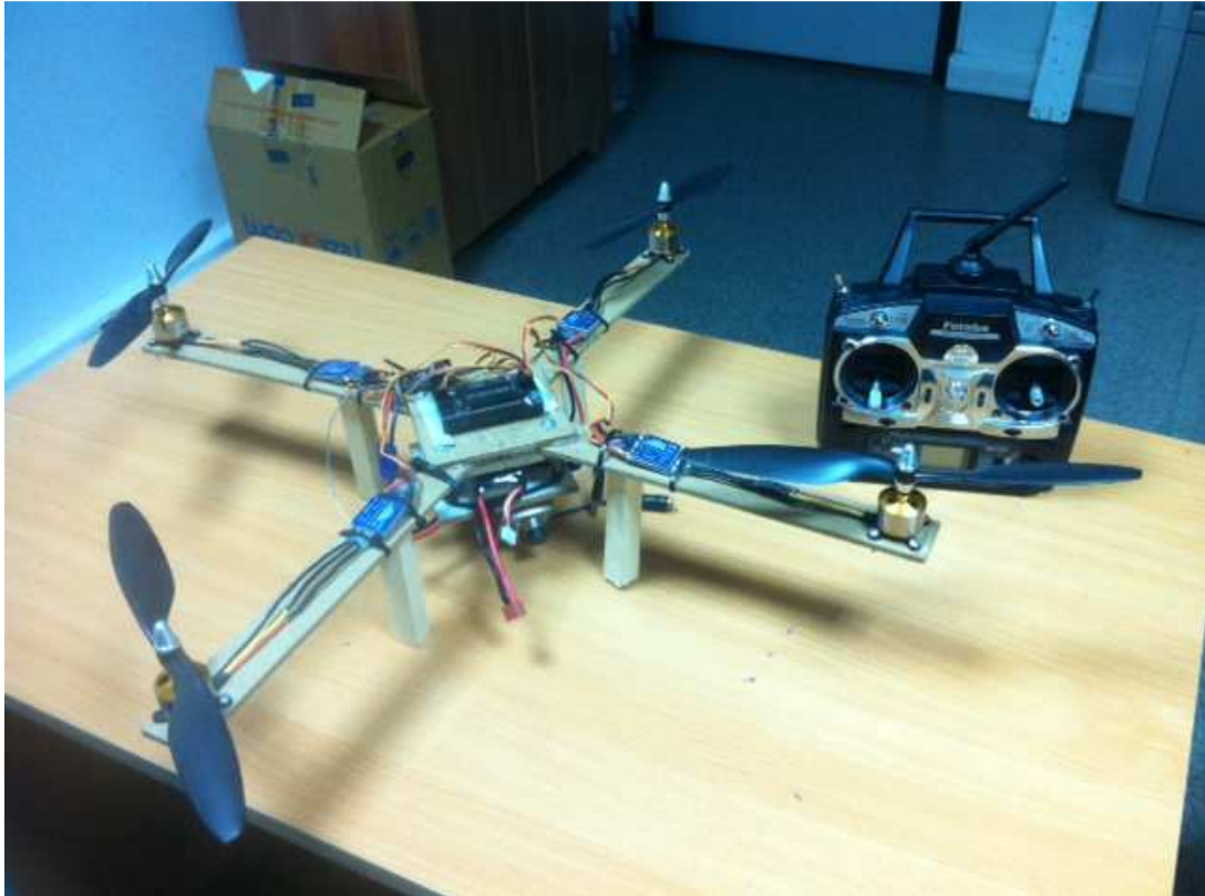
Figure 5.4 The Quadrotor that built in this work and Futaba remote controller
