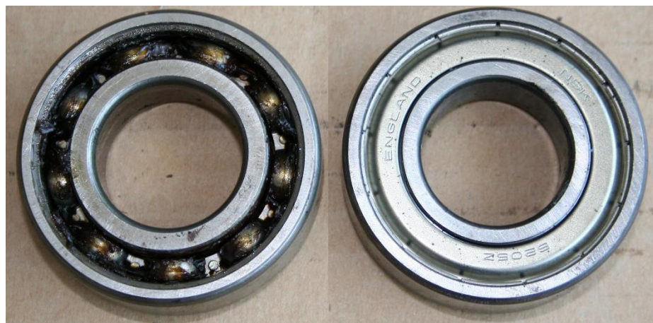
Figure 2.2. Faulty and unused bearings respectively
