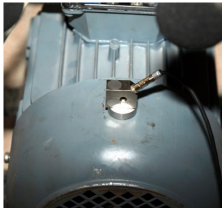
Figure 2.5. Accelerometer and its position
