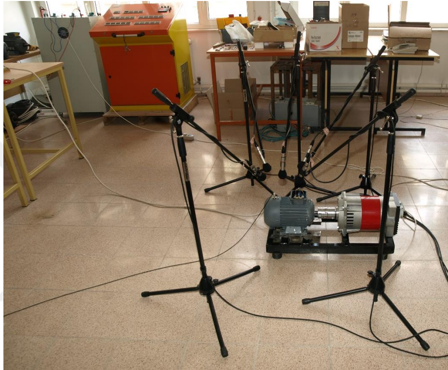
Figure 2.6. Experimental Setup for vibration and acoustic data
