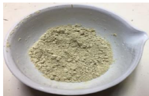
b) Lime-water- calcium lignosulfonate
