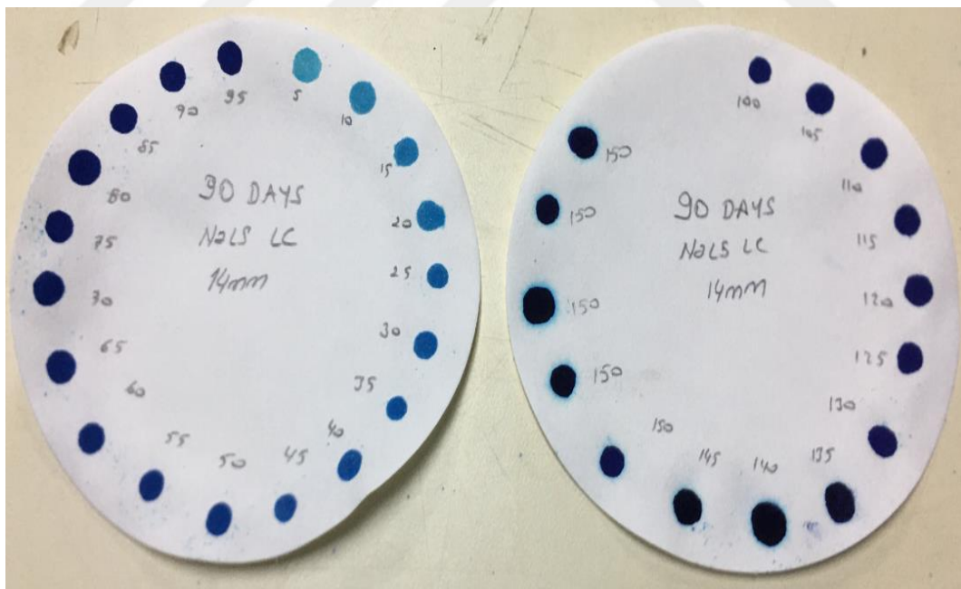
Figure 4.16 Methylene blue test data obtained from NaLS specimen had 14 mm diameter lime column
