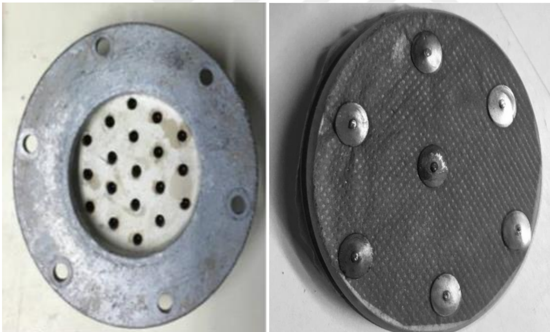
Figure 5.6 The top view of the treated specimens with the CIM stabilization method The first part is that the treated specimen, which has 6.35 cm diameter and 1.9 cm height, was prepared and a free swell test with this specimen was done under 7 kPa and 25 kPa. The swelling potentials of these treated specimens under two surcharge pressures decrease with curing periods that are 1 day, 7 days, 28 days, 90 days, and 180 days. The swelling potentials of these specimens with CIM were illustrated in
