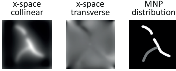
Figure 4.5: Test phantom and the corresponding collinear and transverse images, which are the inputs to the neural networks. The collinear and transverse images correspond the case where the MNP diameter is 25 nm, FOV is 2cmx2cm (i.e., FOV scale = 1), and N_p = 100 .
