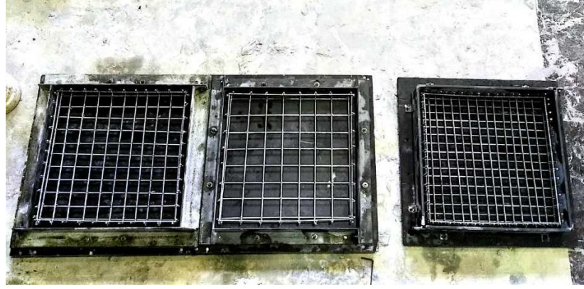
Figure 3.3 Casting mold and reinforcement details.
