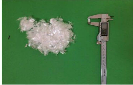
Figure 3.6 Polypropylene (PP) fiber.
