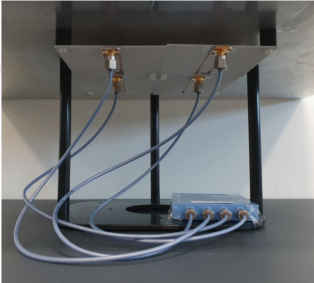
Figure 7.3. Power Divider for Energizing the Antenna with its Connections
