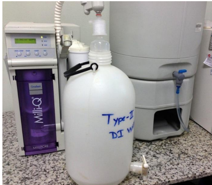
Figure 3.2 Type II DI water supply (Sariavci, 2019)
