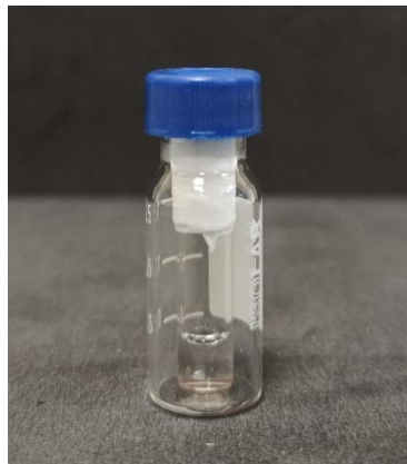
Figure 9. Reaction system used in zeolite synthesis: precursor solution is filled to glass insert, which stays in a glass vial.
