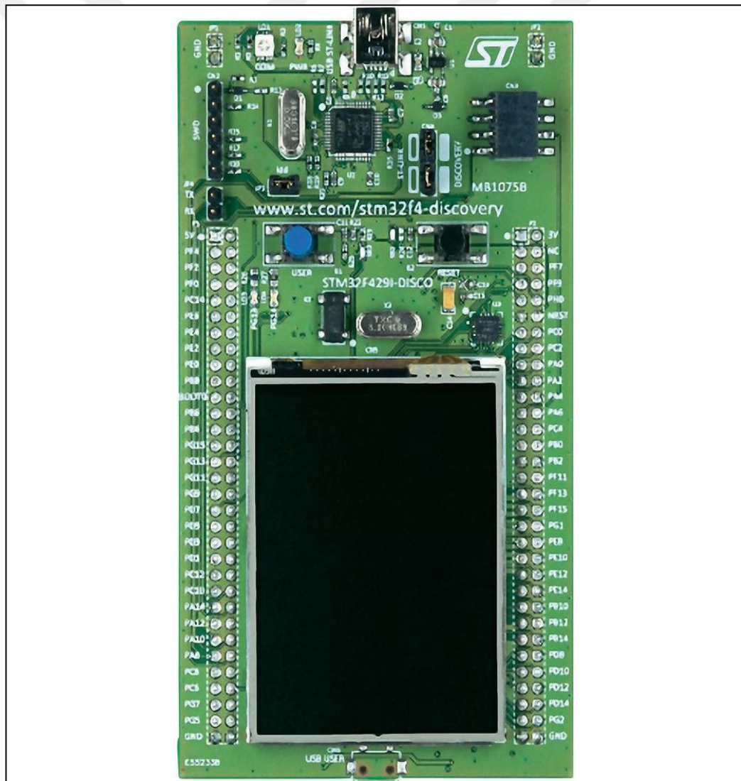
Figure 5.8 STM32F429 Discovery board (ST-STM32F429 Discovery Board, n.d.)
