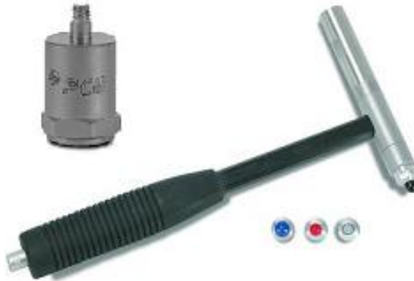
Figure 6.8 Accelerometer and impact hammer for measuring vibration
