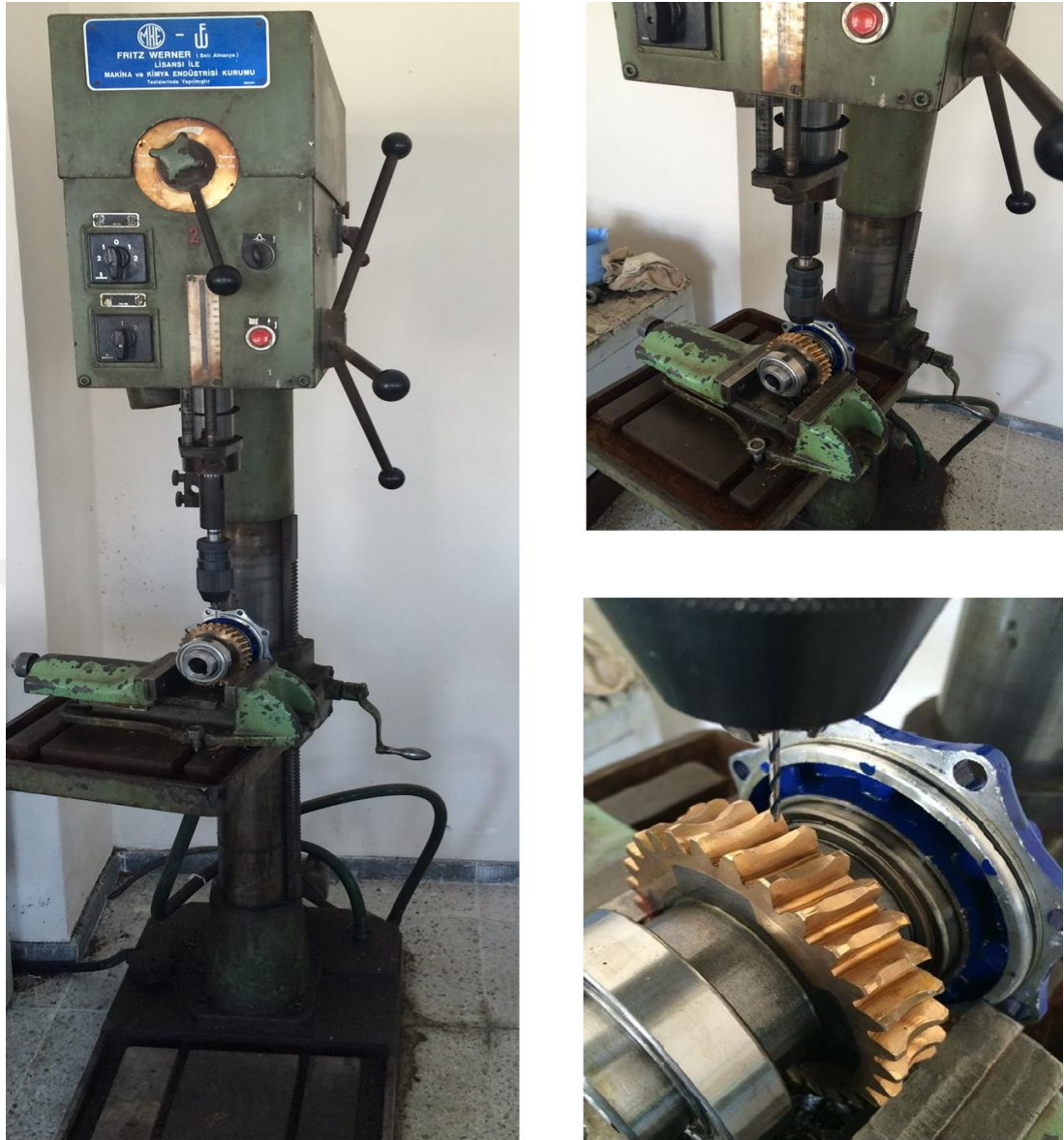
Figure 7.1 Simulated pits with a milling machine
