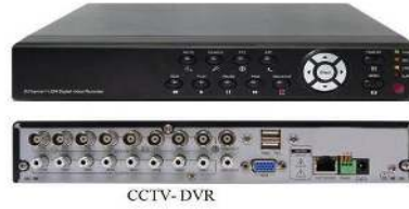
Figure.4. 1CCTV 8 channel DVR device
