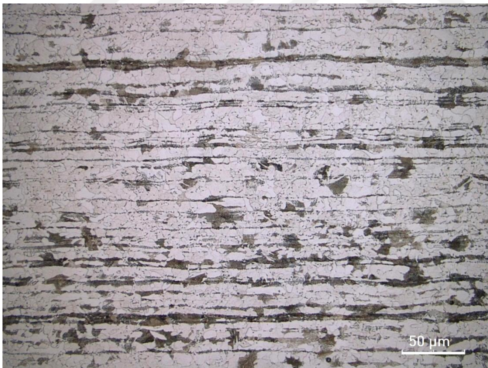
Figure 4.2. Microstructure of Part2. Etched with %2 Nital. Dark regions are pearlite, white regions are ferrite.
