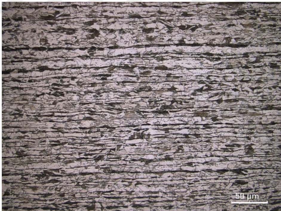
Figure 5.1. Light Microscope image of 680-30-5. Dark regions are pearlite, white regions are ferrite.
