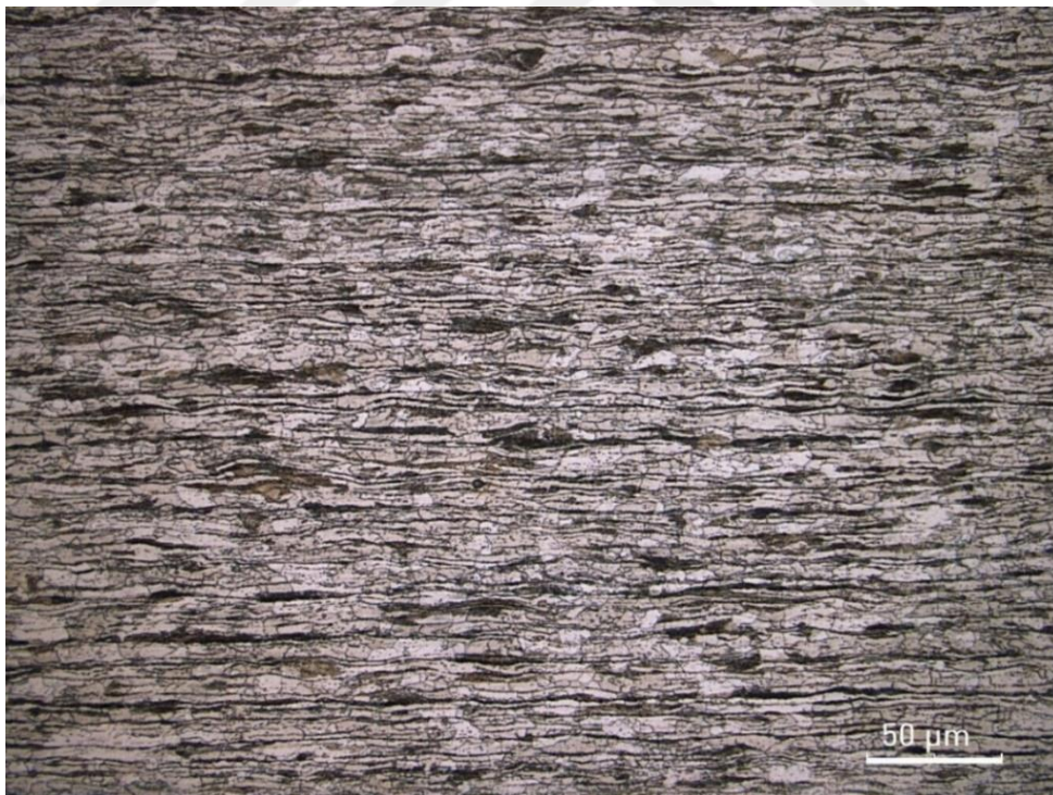
Figure 5.4. Light Microscope image of 680-60-5. Dark regions are pearlite, white regions are ferrite.
