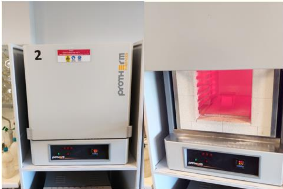
Figure 3.6. Atmospheric heat treatment furnace.
