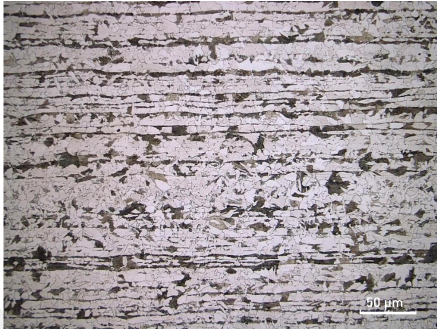
Figure 4.3. Microstructure of Part1. Etched with %2 Nital. Dark regions are pearlite, white regions are ferrite.
