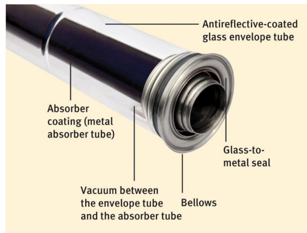
Figure 1.2. The absorber tube with the glass cover [4]
