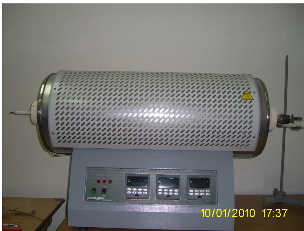
Figure 3.1 Three zone tube furnace
