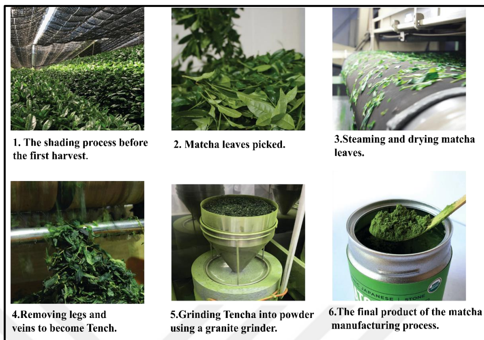
Figure 1.5. Steps of manufacturing MJGT by the Jade Leaf brand
