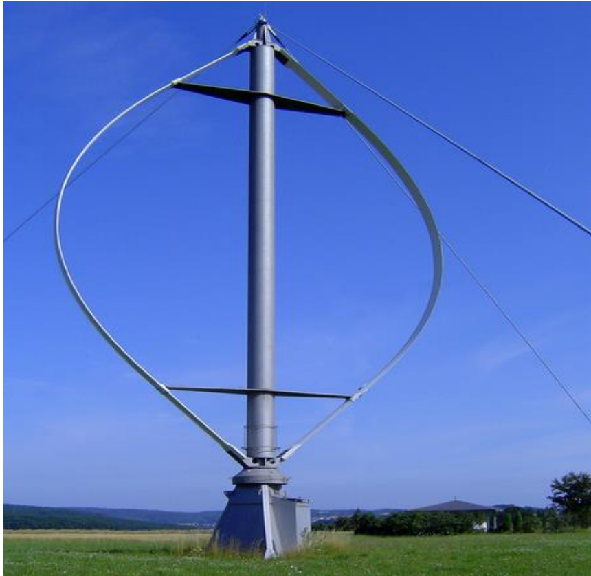
Figure 2.3 : Vertical Axis Wind Turbine.
