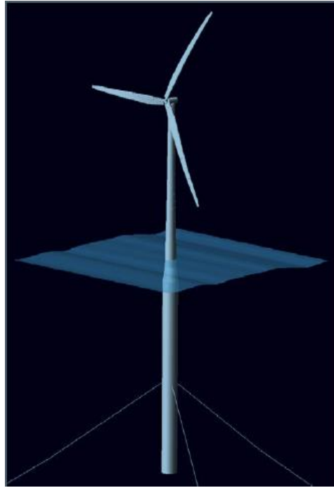
Figure 4.2 : OC3-HyWind platform (Jonkman,2007).
