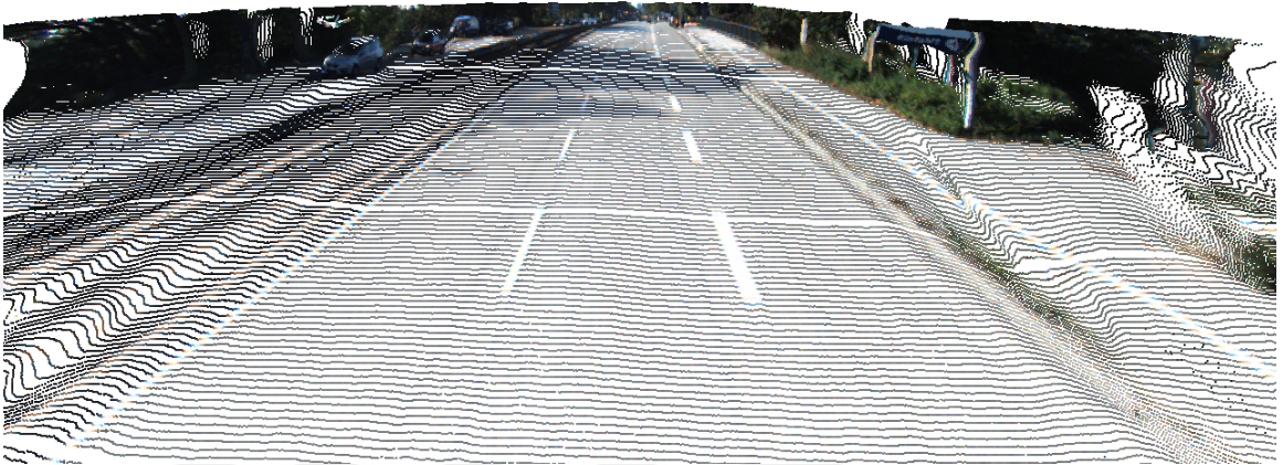
Figure 7: Rendering of pseudo-LiDAR point cloud. Point cloud is generated from RGB image using monocular depth estimator.
