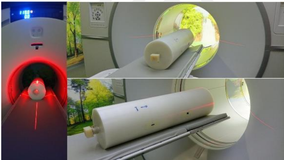
Figure 21. Practical testing of a count performance for the PET scanner
