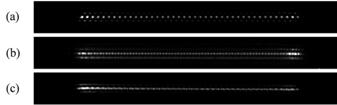
Figure 5.18: Experimental results of the line scans. (a) The MMLA motion only produces discrete addressing; (b) The PSL and the MMLA move synchronously and phase condition is met at all times and continuous addressing is achieved (imperfections in the line is due to slight misalignment of the setup). (c) PSFs at five consecutive diffraction orders
