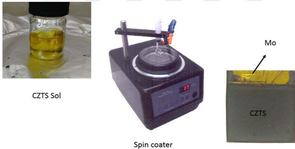
Figure 3.1. CZTS precursor solution, spin coater and CZTS thin film on Mo substrate.
