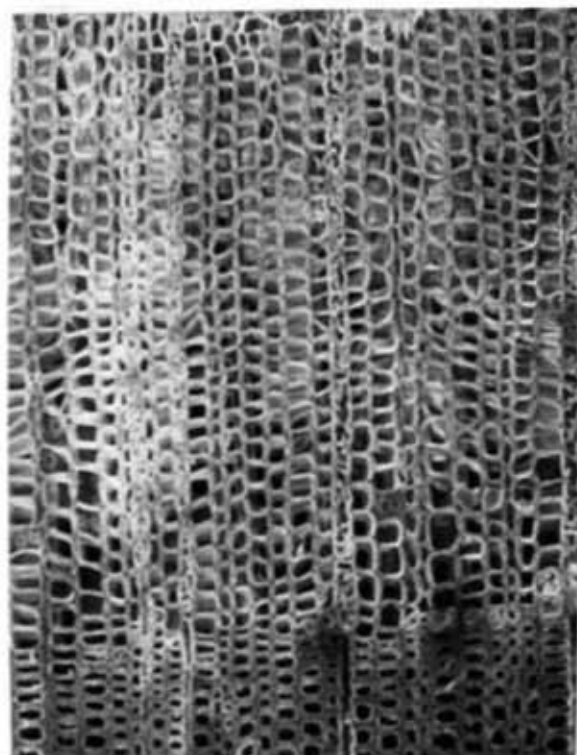
B. Scanning electron micrograph of extreme right portion shown in Fig. 10A. Note border-pitted transverse end walls at different levels within the same radial files. X325
