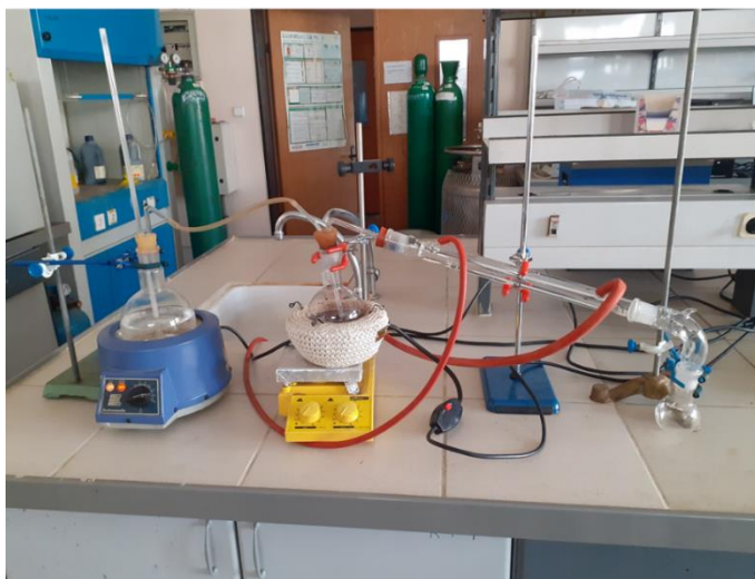
Figure 2.7 Hydrodistillation and evaporation by rotary evaporator (Personal archive, 2021)
