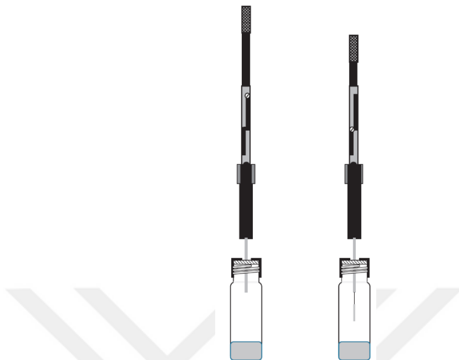
Figure 1.5 Fiber position as up and down positions in headspace-solid phase microextraction (Parker, Elmore, & Balagiannis 2015)
