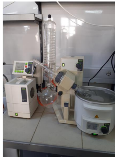
Figure 2.7 Hydrodistillation and evaporation by rotary evaporator (Personal archive, 2021)
