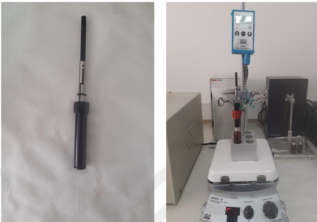
Figure 2.6 Incubation of samples and insertion of the SPME fiber to the sampling vial (Personal archive, 2021)
