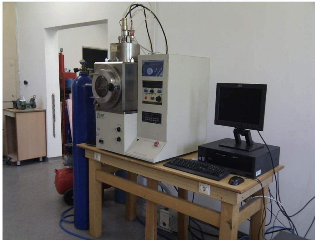
Figure 3. 2: Image of DC Sputter
