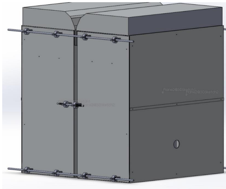
Figure 2.22 : Rods used on cases.
