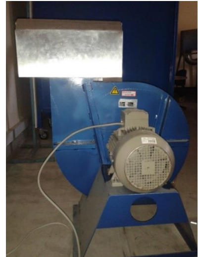
Figure 4.2 : The fan and mounted drawer case on it.
