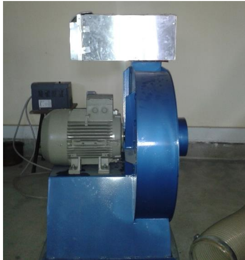
Figure 4.1 : The fan and mounted drawer case on it.
