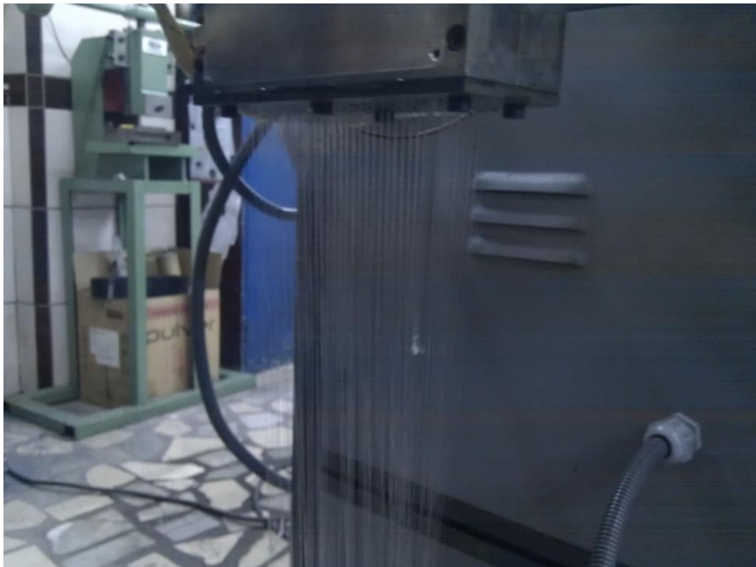
Figure 2.1 : Hot and slenderized polymer coming out of die.
