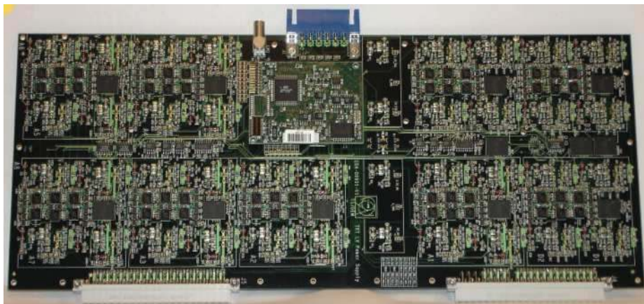
Figure 3.5: Low voltage patch panel board
