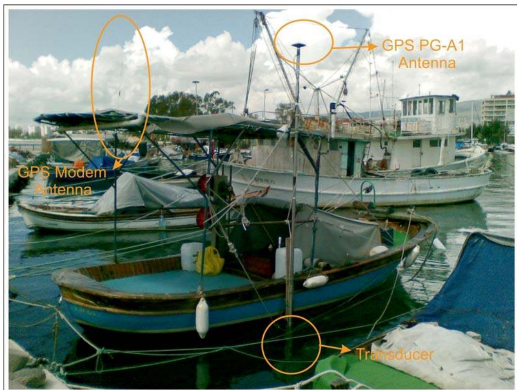
Figure 5.16 GPS modem antenna, GPS PG-A1 antenna, and transducer on the survey vessel
