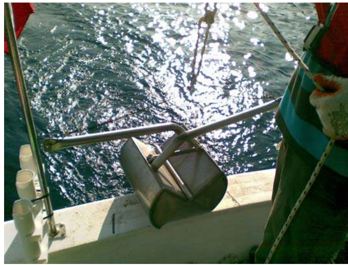
Figure 1.4 Using grab sampler on this study
