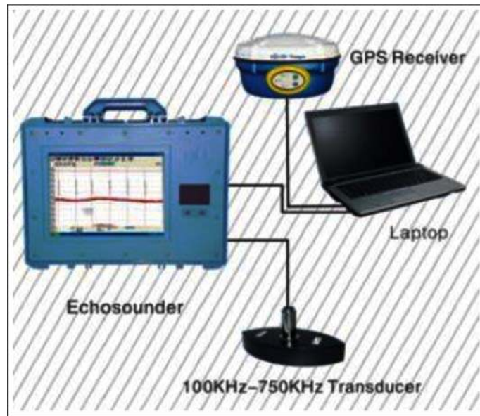
Figure 5.15 Using 200 kHz transducer and work scheme of equipments
