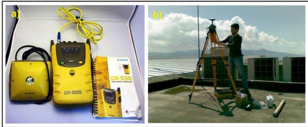
Figure 5.10 a) TopCon GPS GB-500 and b) The installation of the reference station using tripod
