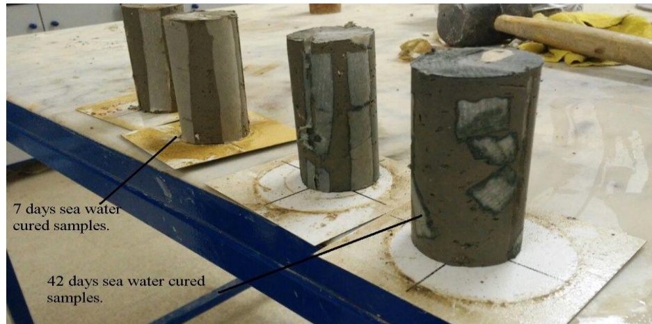
Figure 3.13 Color change in long term sea water curing (Personal archive, 2018)
