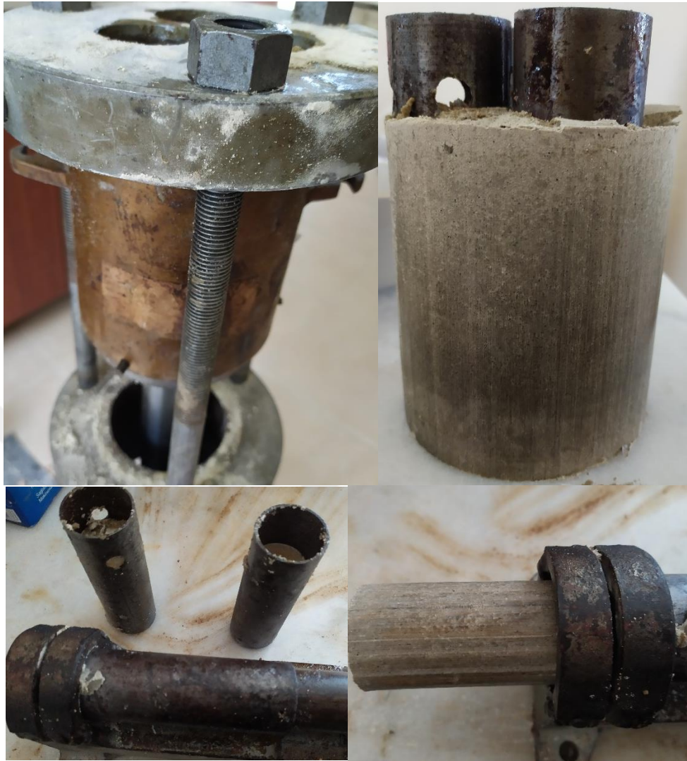
Figure 2.16. Samples preparation for UCS test
