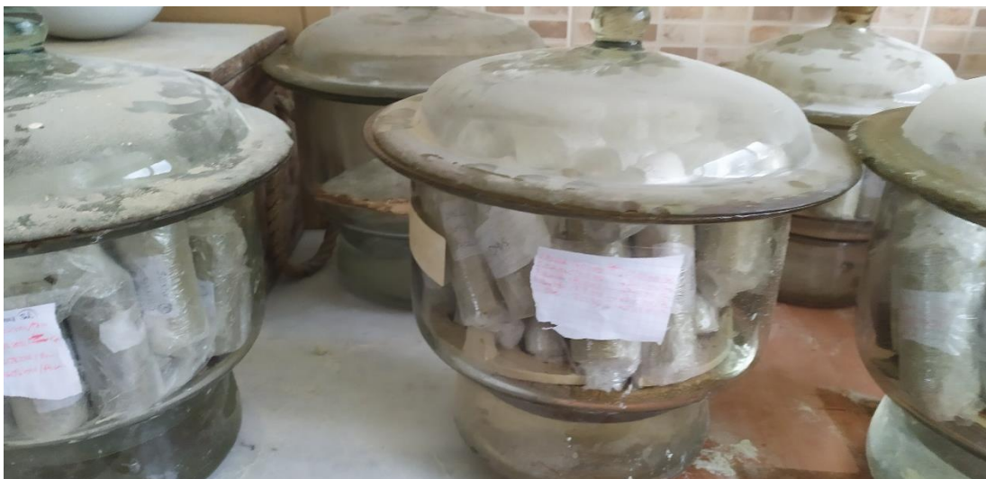
Figure 2.17. Curing of the samples for 1, 7, and 28 days
