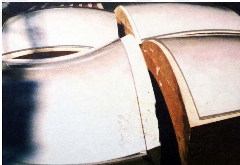
Figure 46. Forming of acrylic-glass elements (Dunn, 2012, p. 152).
