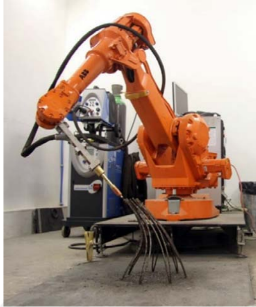
Figure 34. A 6-axis CNC robot arm (Naboni & Paoletti, 2014, p. 72).
