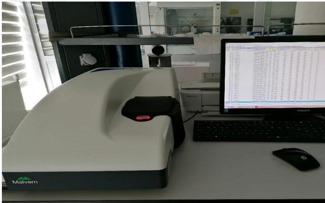
Figure 2. 5 Image of the device where zeta potential and particle size distribution analyses were performed
