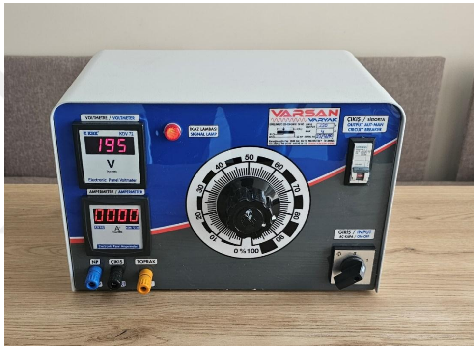
Figure 4.3. The experimentally used autotransformer (variac).
