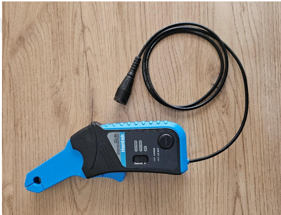
Figure 4.10. The practically used current measurement probe.
