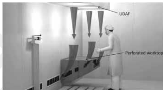
Figure 4. Operator protection in weighing room
