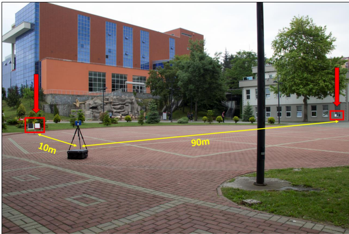
Figure 3.17 Simplified experimental configuration. The black and white plates are marked with red arrows.
