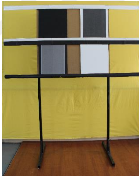
Figure 3.12 The test stand containing the four plates in white, light gray, dark gray and black colors.
